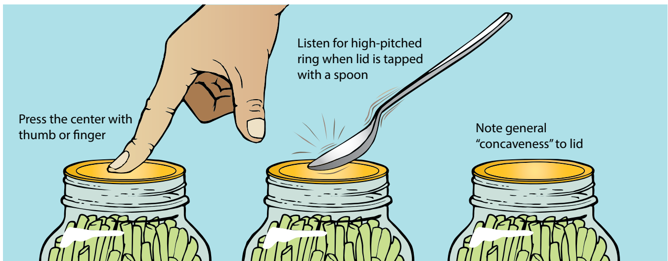
Figure 8. Testing the seal.
