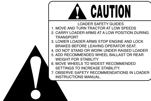
Figure 1. Typical safety sign for front-end loaders.
