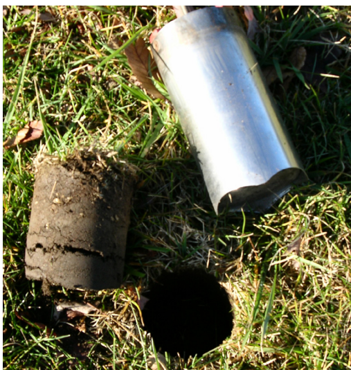
Figure 3. Cutter blade and plug just removed from turf.
