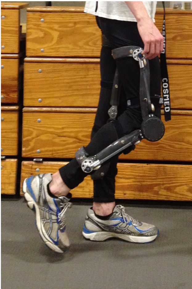
Figure 4: An active knee exoskeleton (Wevolver 2022).
