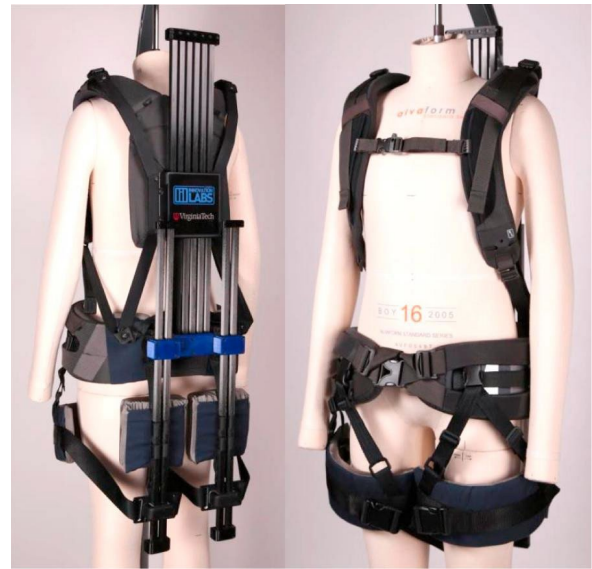
Figure 3: Front and back view of Virginia Tech and Lowe's passive Exoskeleton (Alemei et al. 2019).
