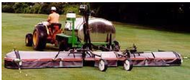
Figure 1. A skirt over a spray boom can virtually eliminate pesticide drift.
