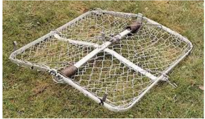
Figure 11. Example of a "suitcase" style of live catch cage trap used to capture beaver. (Reprinted from Chapter 2 of Human Health and Ecological Risk Assessment for the Use of Wildlife Damage Management Methods by U.S. Department of Agriculture's Animal and Plant Health Inspection Service—Wildlife Services, 2019, p. 6, available to download at https://www.aphis.usda.gov/wildlife_damage/nepa/risk_assessment/2-cage-trap-peer-reviewed.pdf .)
