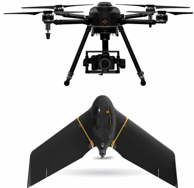
Figure 48: Quadcopter SkyFish M4 and fixed-wing Sensefly eBee drones. (Photos provided by SkyFish and Sensefly.)
