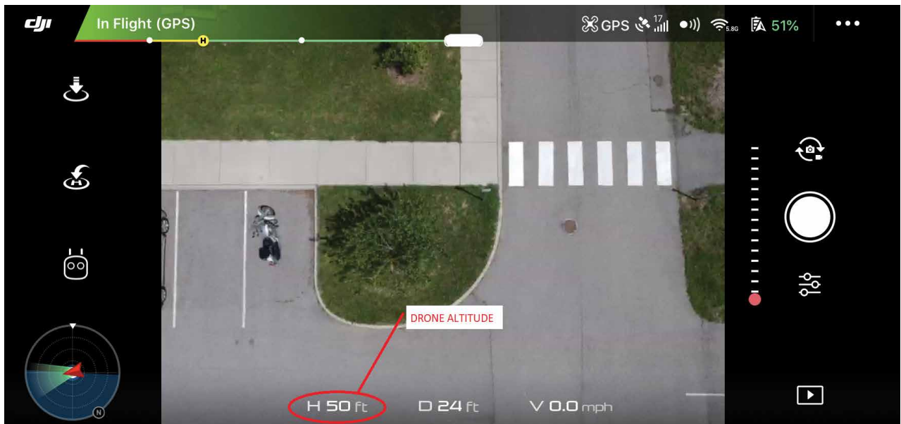
Figure 20: FPV application view showing altitude measurement.
