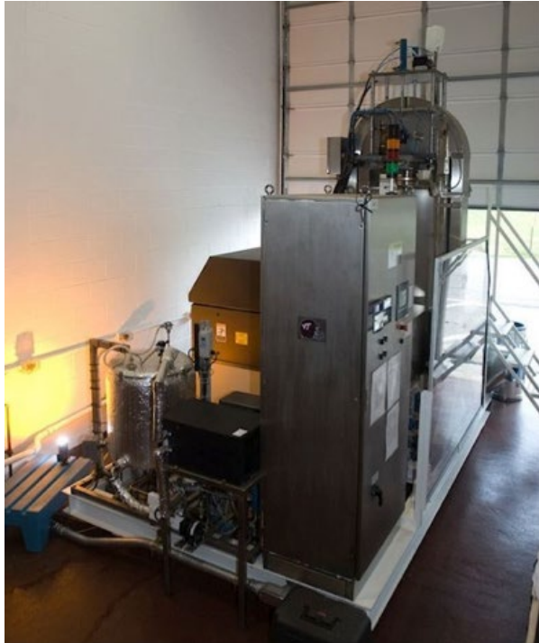
Figure 3. This is a pilot-scale high pressure processor that performs batch processing. (Photo courtesy of Brett Driver, Virginia Tech, Department of Food Science and Technology.)
