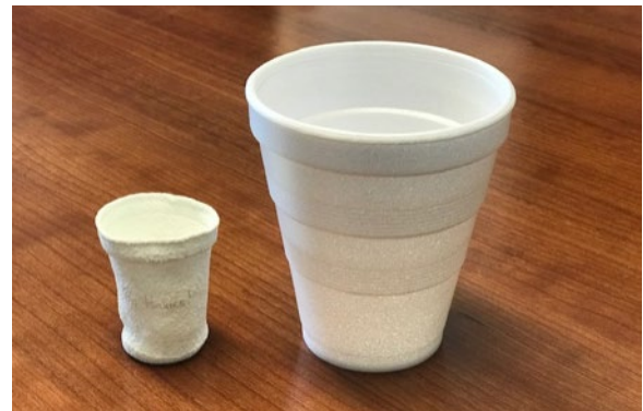
Figure 2. Products that contain a high volume of air, such as plastic foam cups, shrink after being exposed to HPP. (Photo courtesy of Nicole Arnold, Virginia Tech.)
